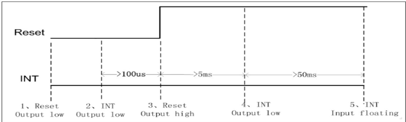
Figure 7.4: Setting Slave Address to 0xBA/0xBB Timing
