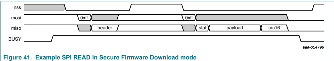
Figure 41. Example SPI READ in Secure Firmware Download mode
