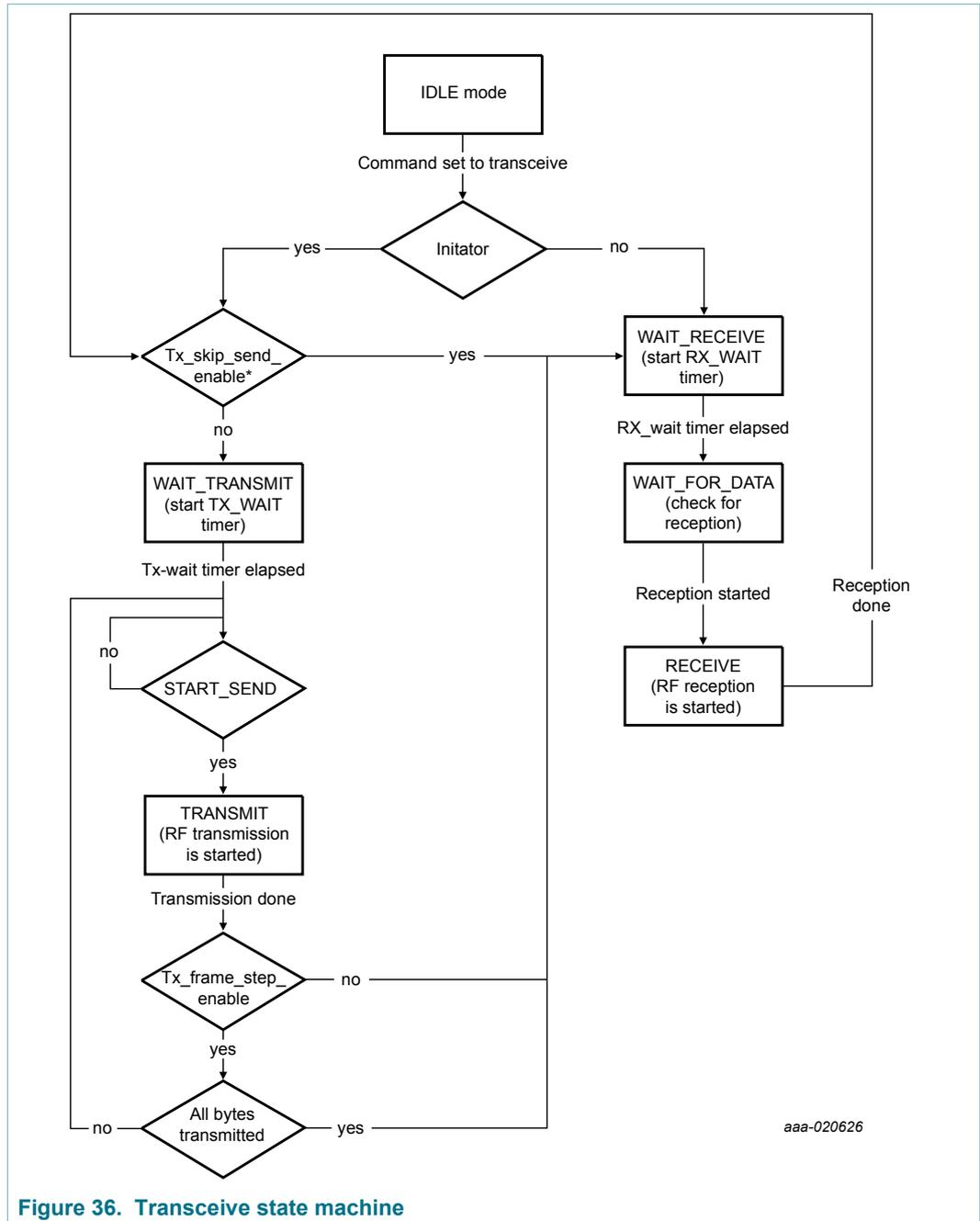
Figure 36. Transceive state machine
