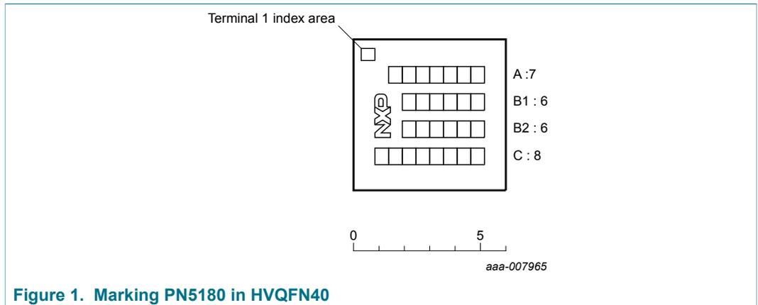
Figure 1. Marking PN5180 in HVQFN40
