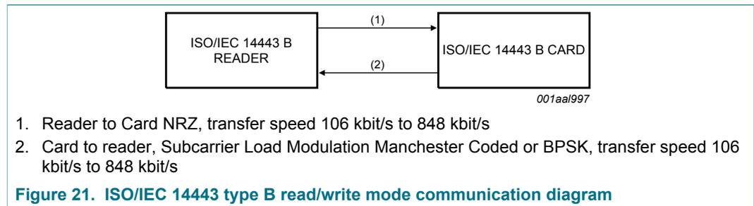
Figure 21. ISO/IEC 14443 type B read/write mode communication diagram
