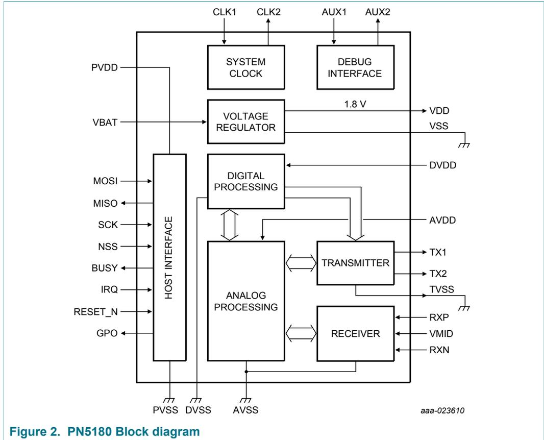
Figure 2. PN5180 Block diagram
