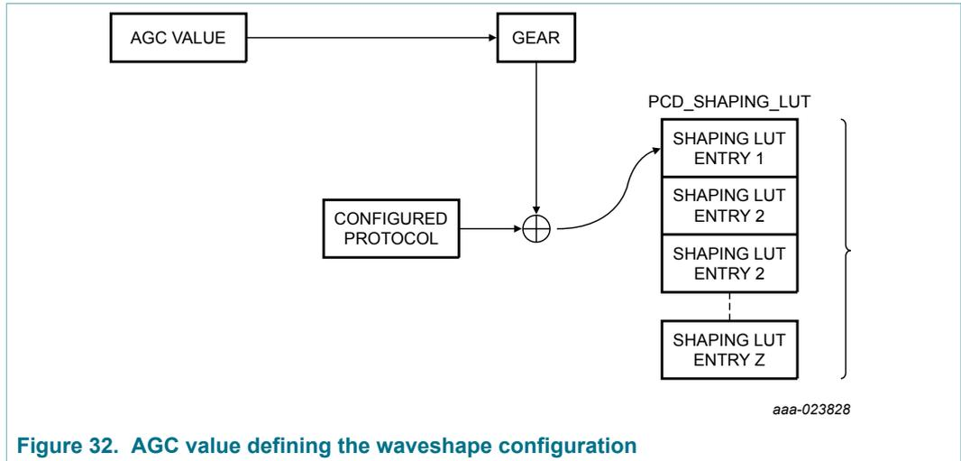
Figure 32. AGC value defining the waveshape configuration
