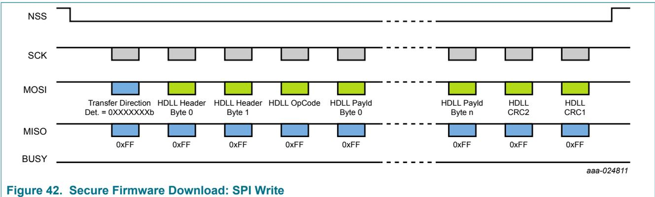
Figure 42. Secure Firmware Download: SPI Write
