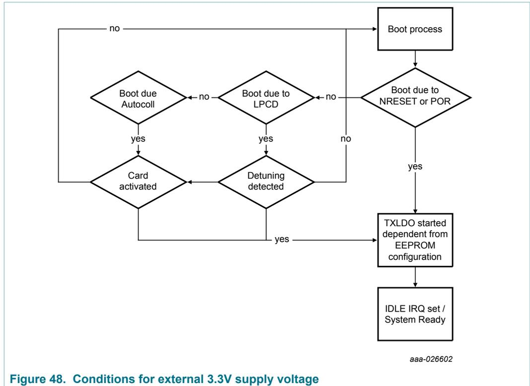
Figure 48. Conditions for external 3.3V supply voltage
