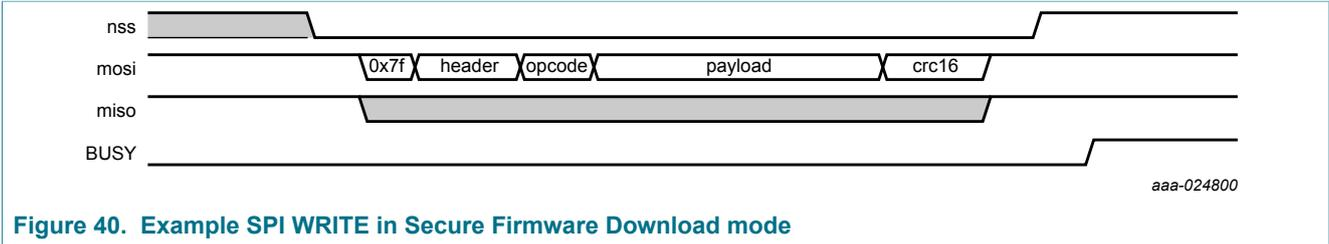
Figure 40. Example SPI WRITE in Secure Firmware Download mode
