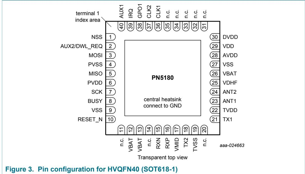
Figure 3. Pin configuration for HVQFN40 (SOT618-1)
