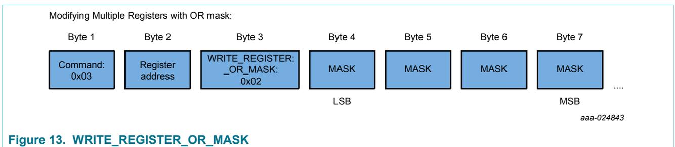
Figure 13. WRITE\_REGISTER\_OR\_MASK
