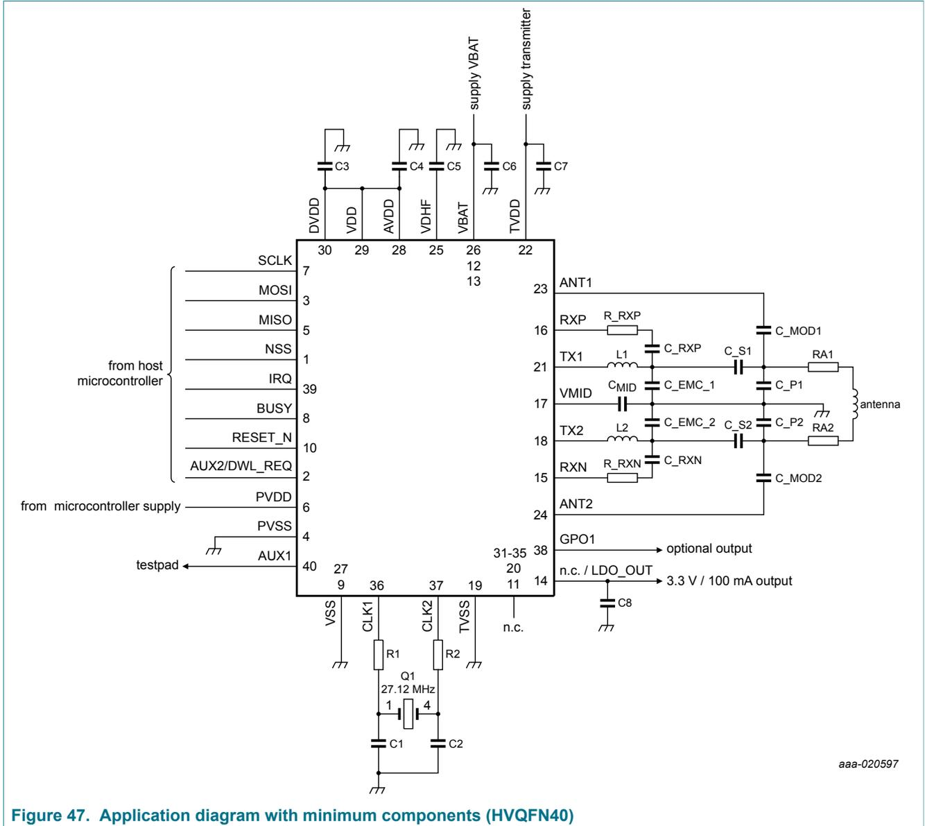
Figure 47. Application diagram with minimum components (HVQFN40)
