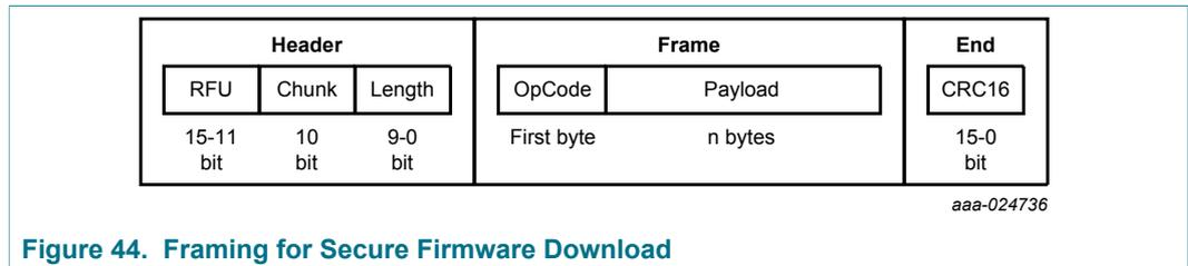
Figure 44. Framing for Secure Firmware Download
