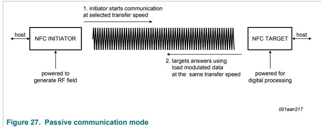
Figure 27. Passive communication mode
