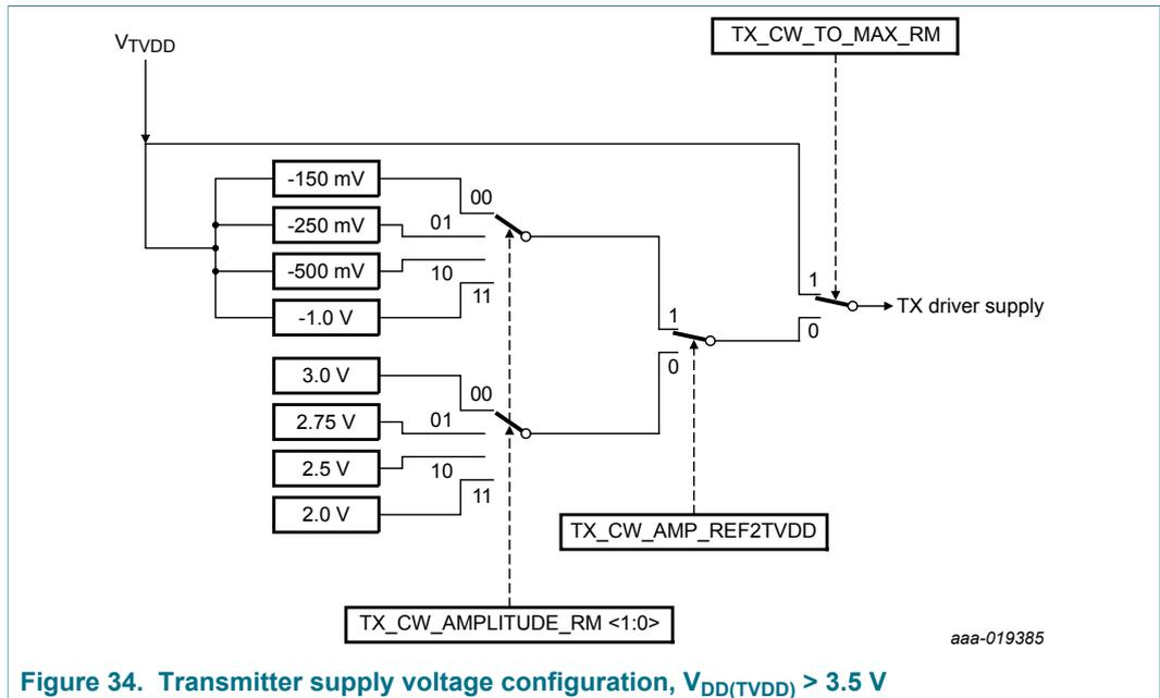
Figure 34. Transmitter supply voltage configuration,  $V_{DD(TVDD)} > 3.5 V$
