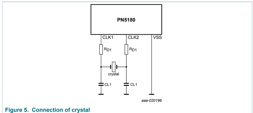
Figure 5. Connection of crystal
