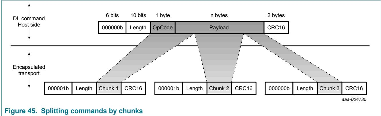
Figure 45. Splitting commands by chunks
