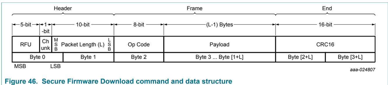
Figure 46. Secure Firmware Download command and data structure
