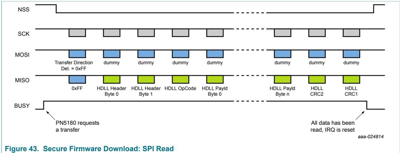
Figure 43. Secure Firmware Download: SPI Read
