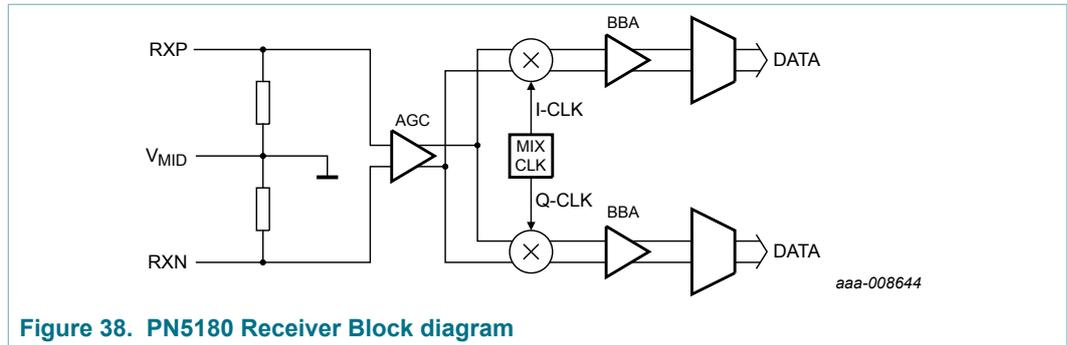
Figure 38. PN5180 Receiver Block diagram
