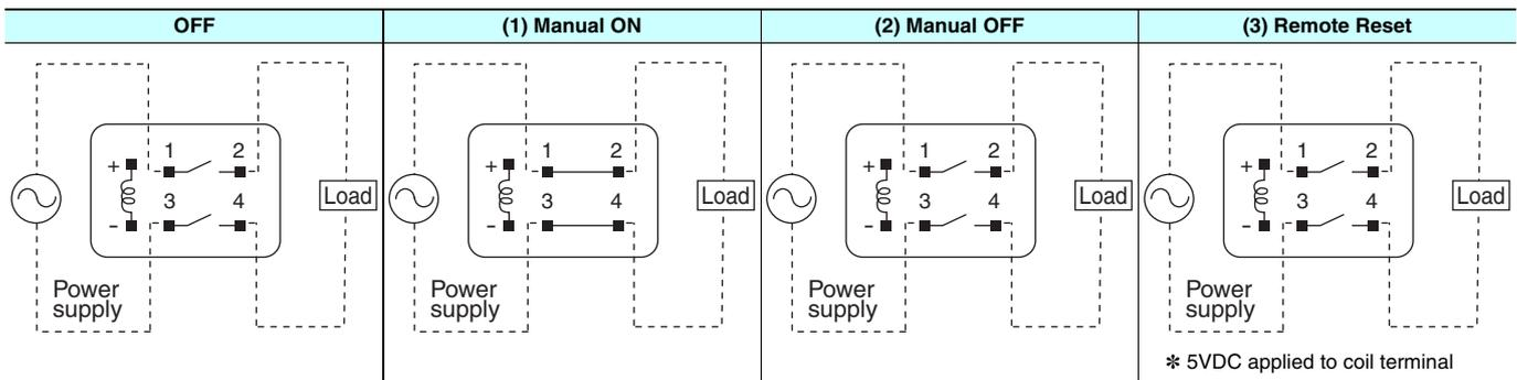
Note: 1. The above circuit is referring to the 'A8GS-Dxxxx' model.
