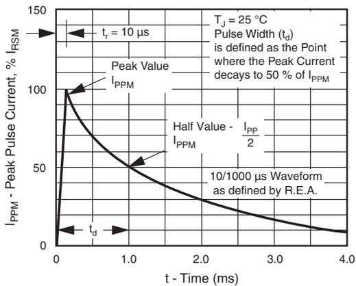
Fig. 3 - Pulse Waveform
