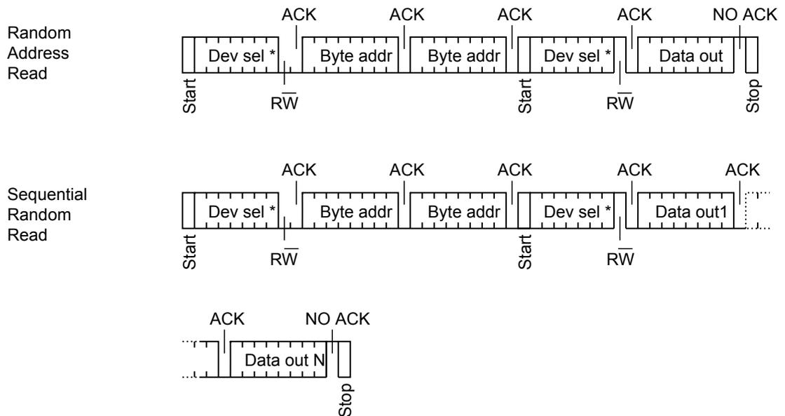
\*: The seven most significant bits of the device select code of a random read must be identical.
