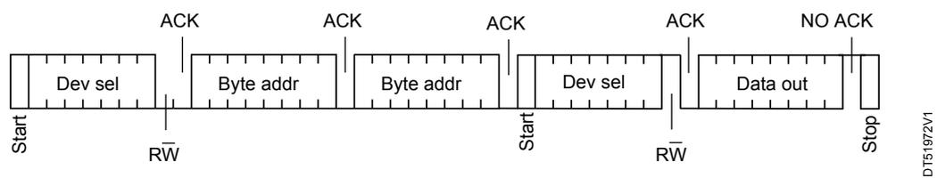
\* The seven most significant bits of the first device select code of a random read must be identical to the seven most significant bits of the second device select code
