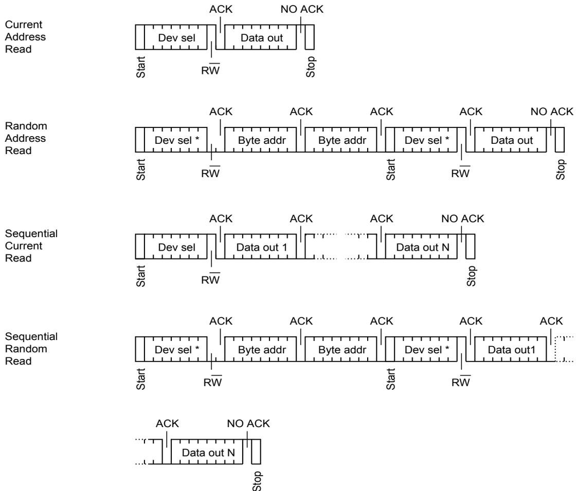
**Note:** The seven most significant bits of the first device select code of a random read must be identical to the seven most significant bits of the device select code of the write.
