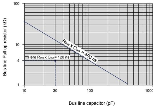
The  $R_{bus} \times C_{bus}$  time constant must be below the 400 ns time constant line represented on the left
