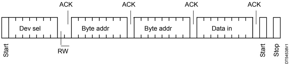
**Figure 14. Read lock status with identification page locked**
