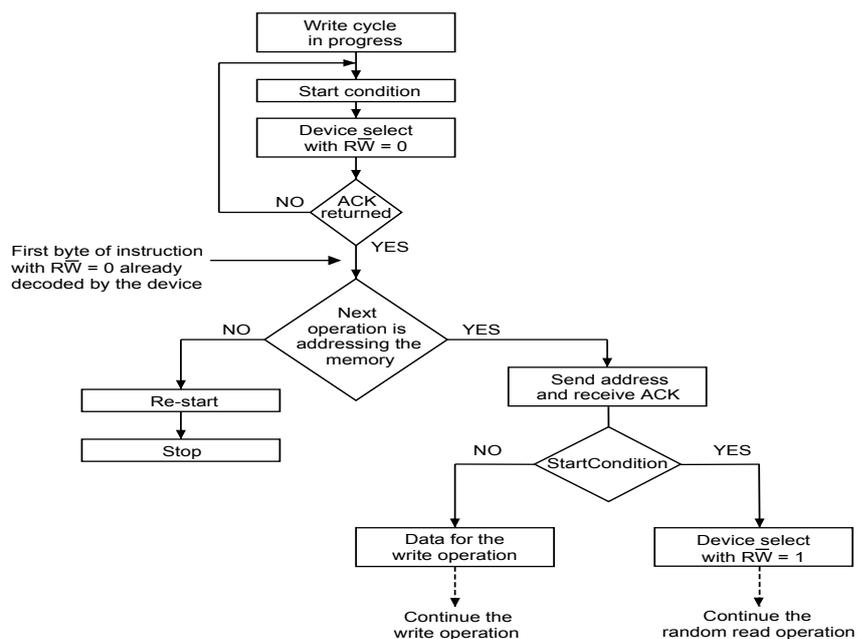
*Note:* The seven most significant bits of the device select code of a random read (bottom right box in the [Figure 8](#)) must be identical to the seven most significant bits of the device select code of the write (polling instruction in the [Figure 8](#)).
