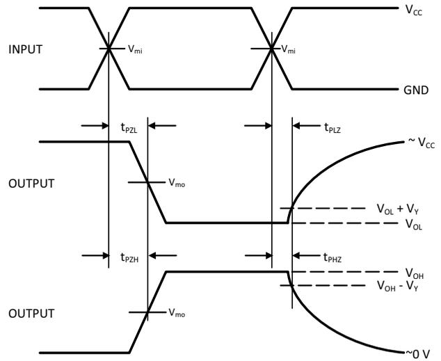
**Figure 4. Switching Waveforms**
