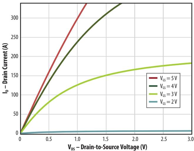
Figure 2: Transfer Characteristics
