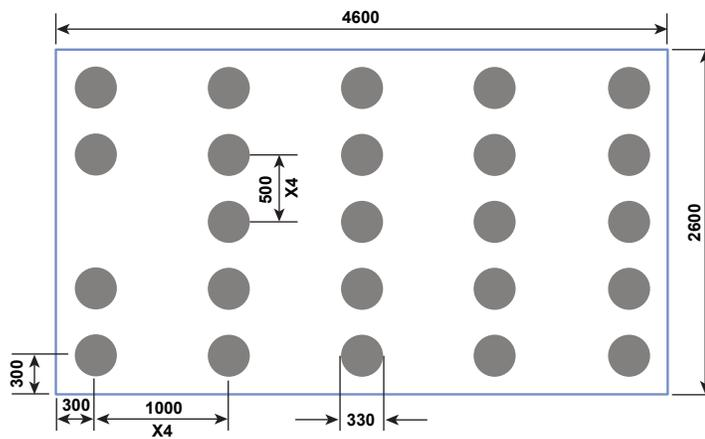
Recommended stencil should be 4mil (100  $\mu\text{m}$ ) thick, must be laser cut, openings per drawing.
