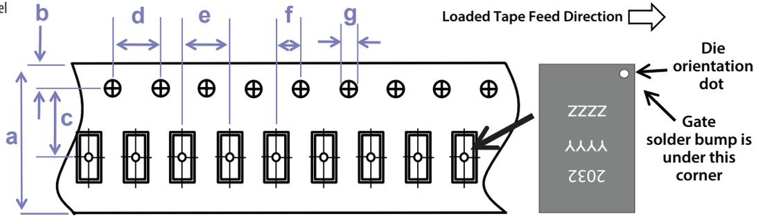
Die is placed into pocket solder bump side down (face side down)
