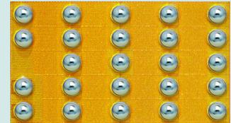
EPC2032 eGaN® FETs are supplied only in passivated die form with solder bumps. Die Size: 4.6 mm x 2.6 mm
