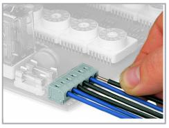
Inserting a solid conductor via push-in termination.
