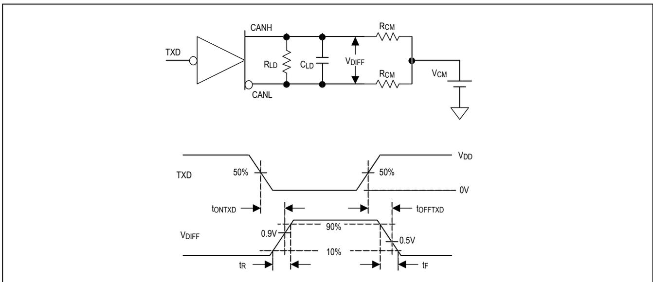
Figure 1. Transmitter Test Circuit and Timing Diagram
