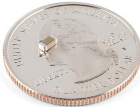
*4.7  $\mu\text{F}$  capacitor on a quarter for size comparison.*
