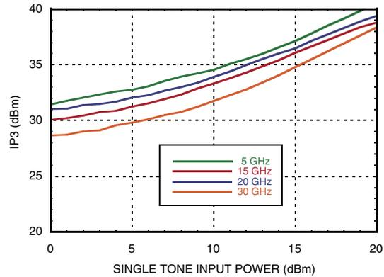
**Input IP3 vs. Input Power Over Temperature**
