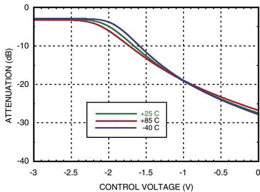
**Attenuation vs. Input Power over Vctrl**
