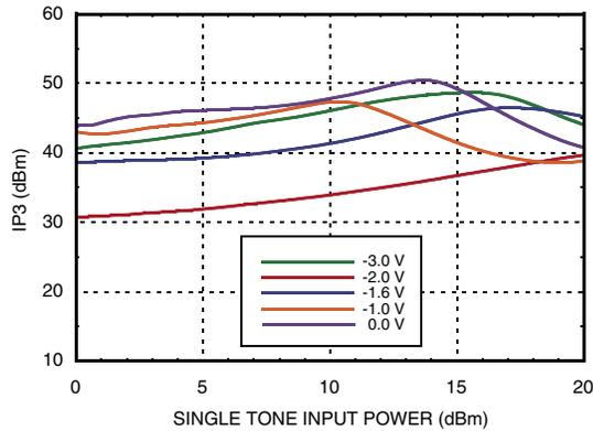
**Input IP3 vs. Input Power Over Frequency**
