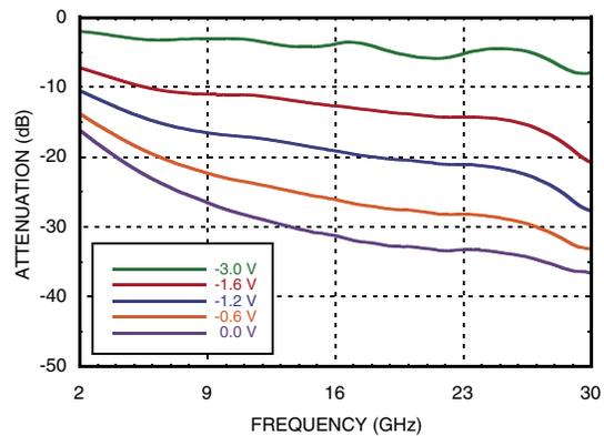
**Attenuation vs. Vctrl over Temperature**
