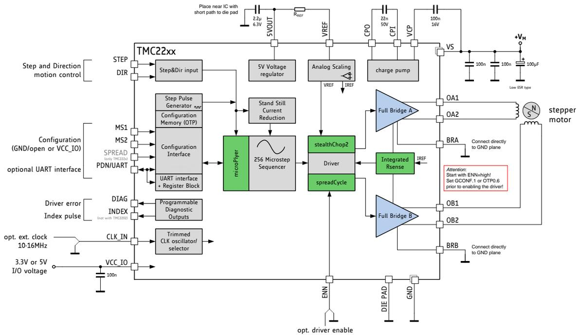
Figure 3.2 Application circuit using RDSon based sensing
