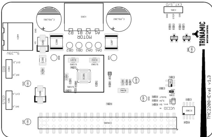
The TMC22xx-EVAL is part of TRINAMICs universal evaluation board system which provides a convenient handling of the hardware as well as a user-friendly software tool for evaluation. The TMC22xx evaluation board system consists of three parts: LANDUNGSBRÜCKE (base board), ESELSBRÜCKE (connector board with test points), and TMC22xx-EVAL.
