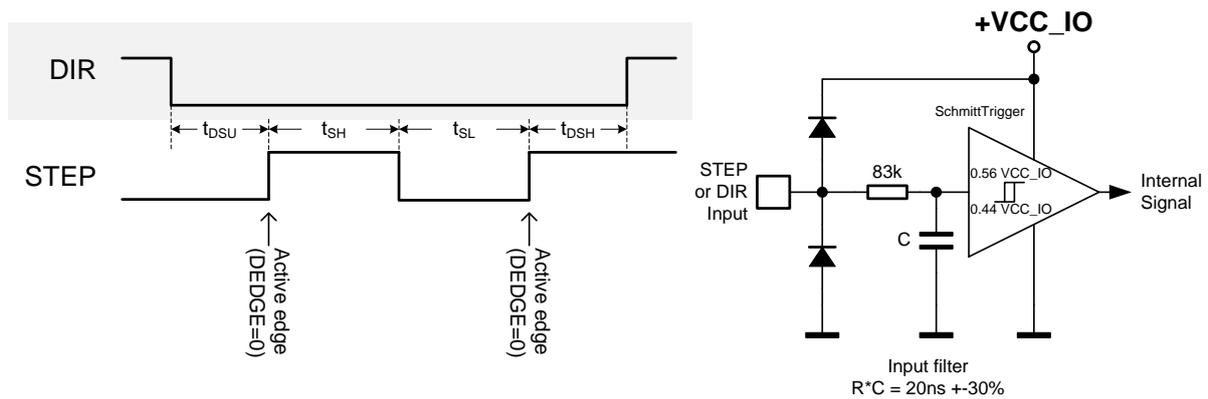
Figure 11.1 STEP and DIR timing, Input pin filter
