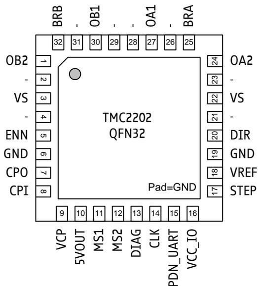
Figure 2.2 TMC2202 Pinning Top View – type: QFN32, 5x5mm<sup>2</sup>, 0.5mm pitch
