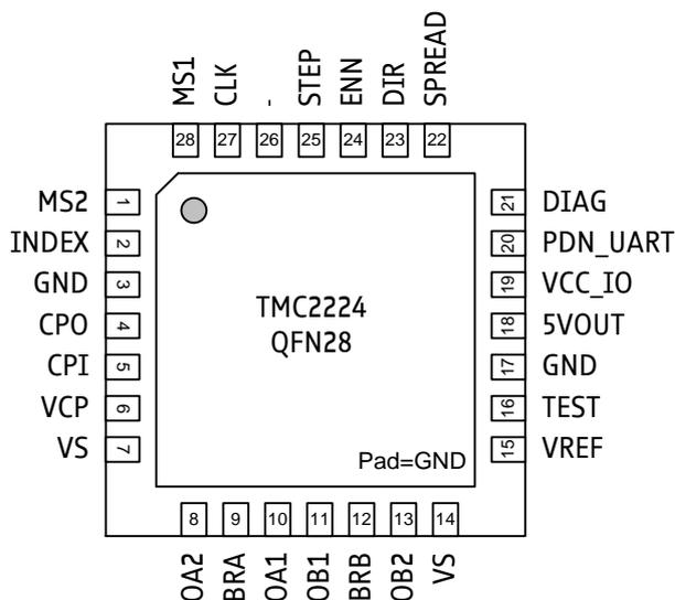
Figure 2.3 TMC2224 Pinning Top View – type: QFN28, 5x5mm<sup>2</sup>, 0.5mm pitch
