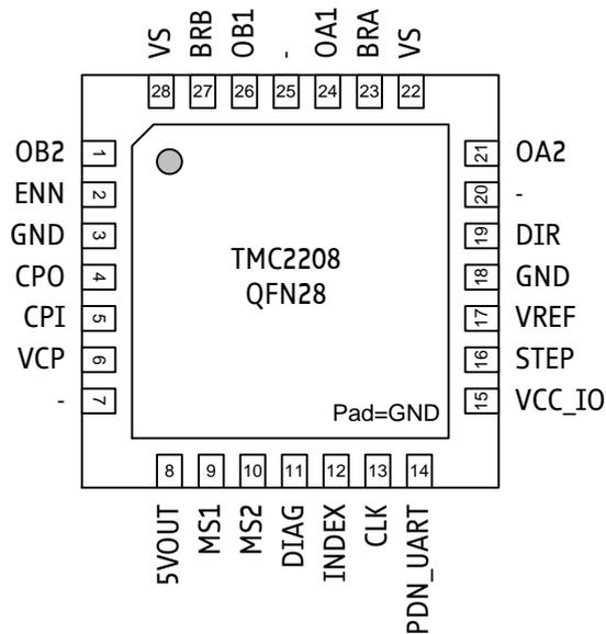
Figure 2.1 TMC2208 Pinning Top View – type: QFN28, 5x5mm<sup>2</sup>, 0.5mm pitch
