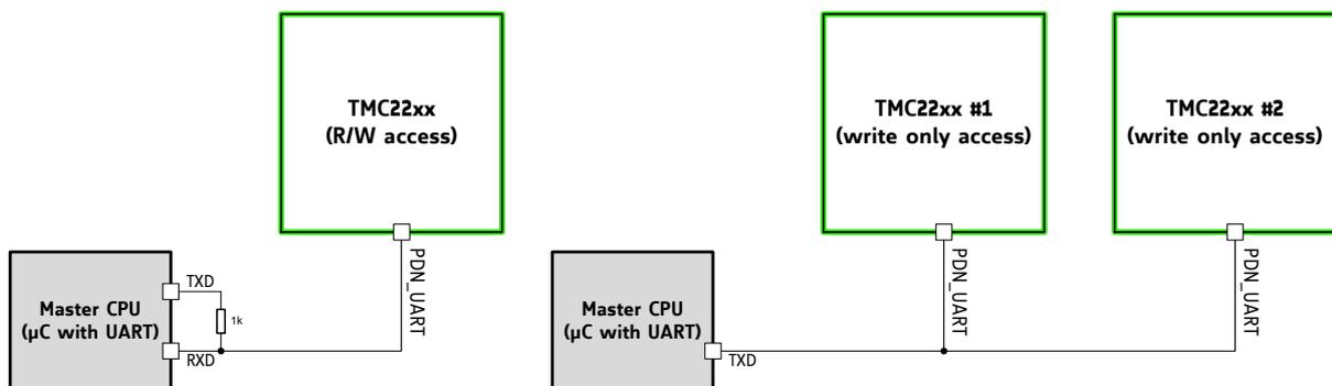
Figure 4.1 Attaching the TMC22xx to a microcontroller UART
