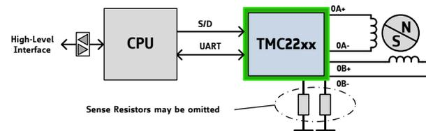
A CPU operates the driver via step and direction signals. It accesses diagnostic information and configures the TMC22xx via the UART interface. The CPU manages motion control and the TMC22xx drives the motor and smoothens and optimizes drive performance.
