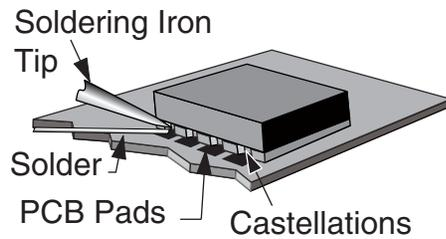
Figure 38: Soldering Technique
