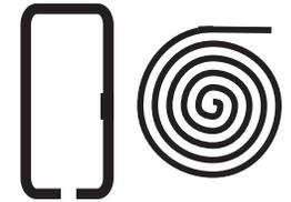
Figure 47: Loop or Trace Antenna
