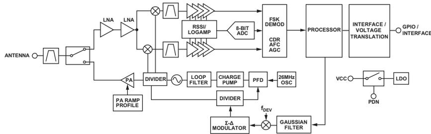
Figure 20: TT Series Transceiver RF Section Block Diagram
