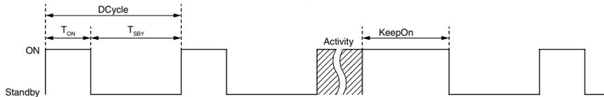
Figure 24: Receiver Duty Cycle
