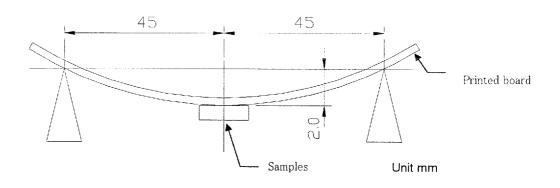
Single sided printed board: glassfabric base, epoxy resin (0.8t, Copper leaf 35um)
