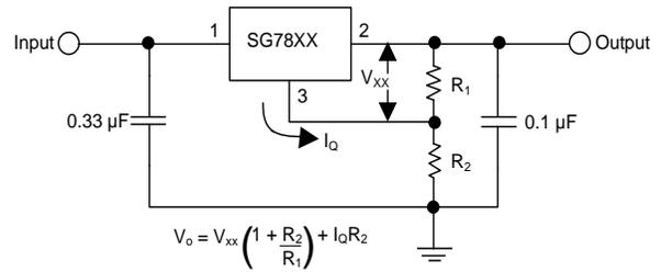
**Figure 6** - Circuit for Increasing Output Voltage
