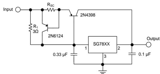
**Figure 7** - High Output Current, Short Circuit Protected
