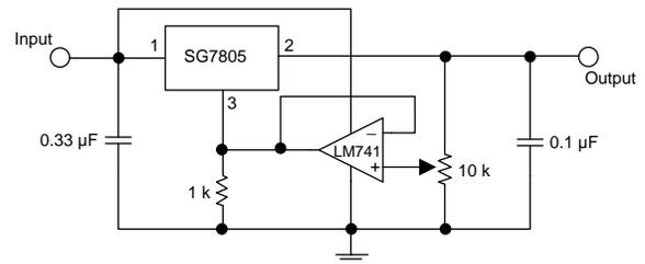
**Figure 8** - Adjustable Output Regulator, 7 V to 30 V
