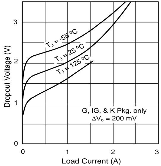
**Figure 3** - Minimum Input-Output Voltage versus Load Current
