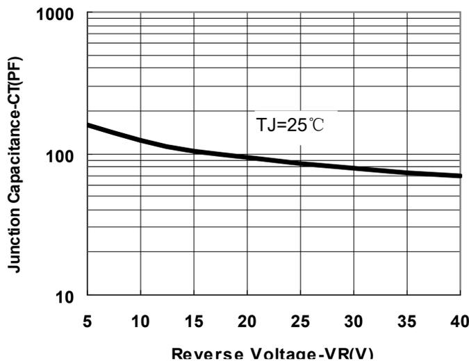
Fig.1-Typical Junction Capacitance
