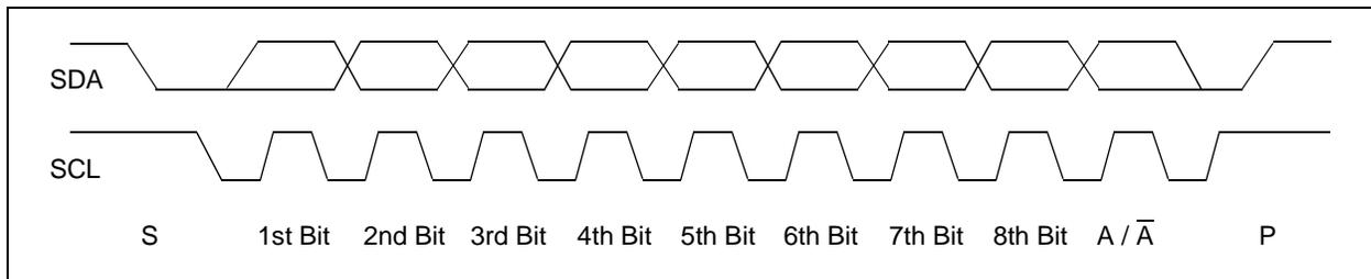
**FIGURE 6-7:** Typical 8-Bit I<sup>2</sup>C Waveform Format.
