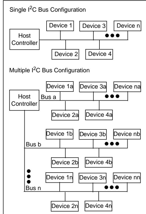
**FIGURE 8-3:** Typical Application I<sup>2</sup>C Bus Configurations.
