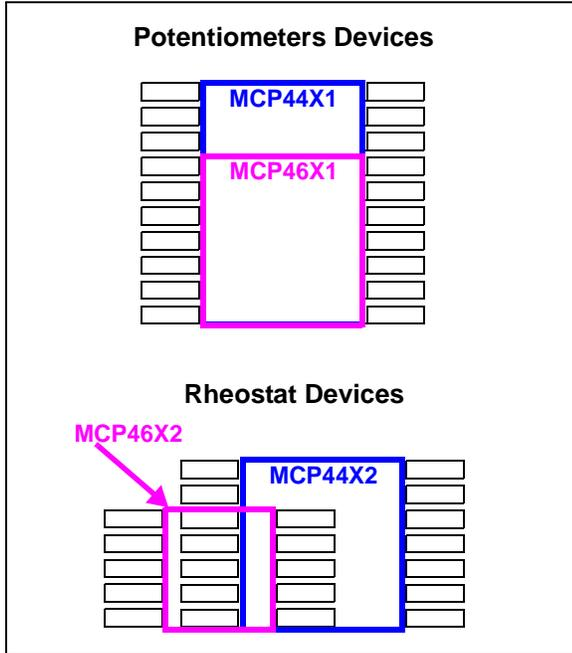
**FIGURE 8-8:** Layout to Support Quad and Dual Devices.
