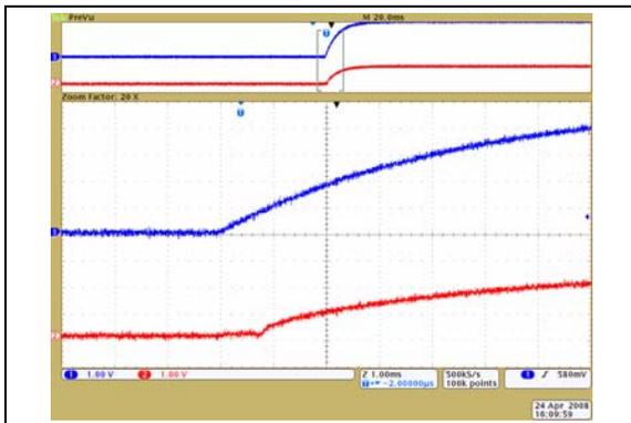
**FIGURE 2-25:** 10 k $\Omega$  – Power-Up Wiper Response Time (1  $\mu\text{s}/\text{Div}$ ).
