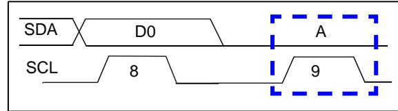
**FIGURE 6-4:** Acknowledge Waveform.
