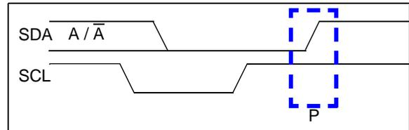
**FIGURE 6-6:** Stop Condition Receive or Transmit Mode.
