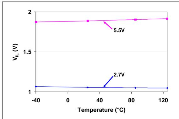
**FIGURE 2-54:**  $V_{IL}$  (SDA, SCL) vs.  $V_{DD}$  and Temperature.
