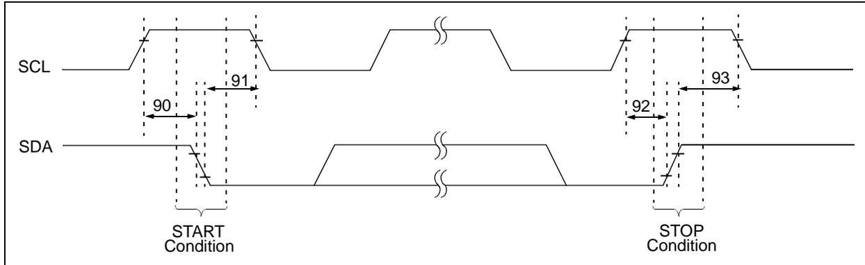
**FIGURE 1-1:** I<sup>2</sup>C Bus Start/Stop Bits Timing Waveforms.
