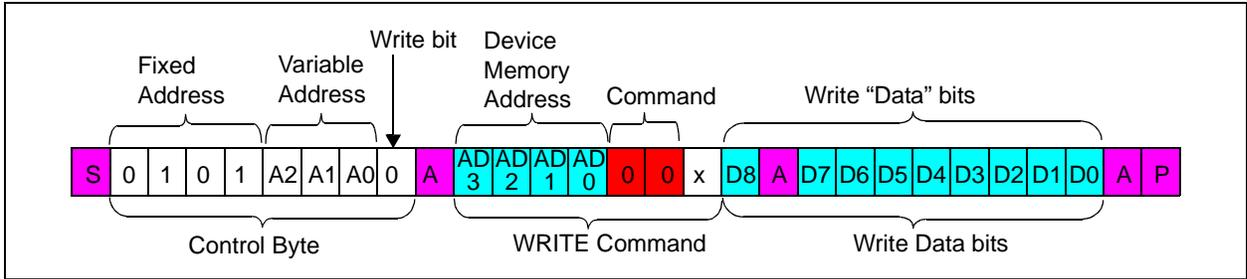
**FIGURE 7-2:** I<sup>2</sup>C Write Sequence.
