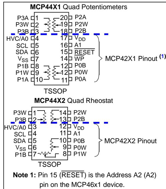
**FIGURE 8-7:** Quad Pinout (TSSOP Package) vs. Dual Pinout.
