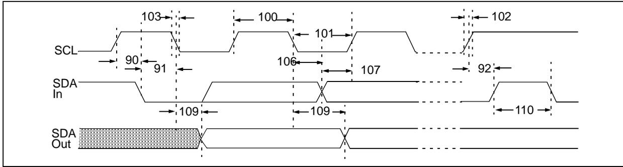
**FIGURE 1-2:** I<sup>2</sup>C Bus Data Timing.
