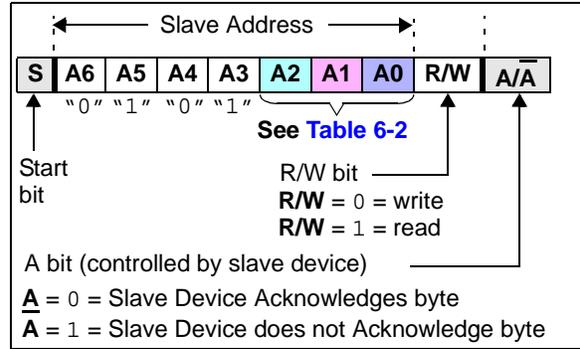
FIGURE 6-9: Slave Address Bits in the I<sup>2</sup>C Control Byte.
