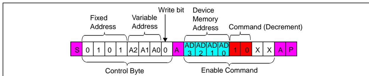
**FIGURE 7-10:** I<sup>2</sup>C Enable Command Sequence.
