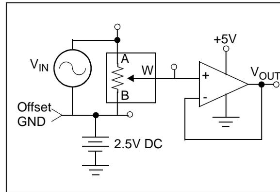
**FIGURE 2-58:** -3 db Gain vs. Frequency Test.
