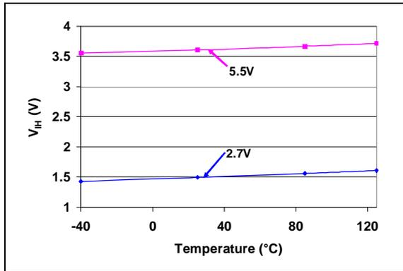
**FIGURE 2-53:**  $V_{IH}$  (SDA, SCL) vs.  $V_{DD}$  and Temperature.
