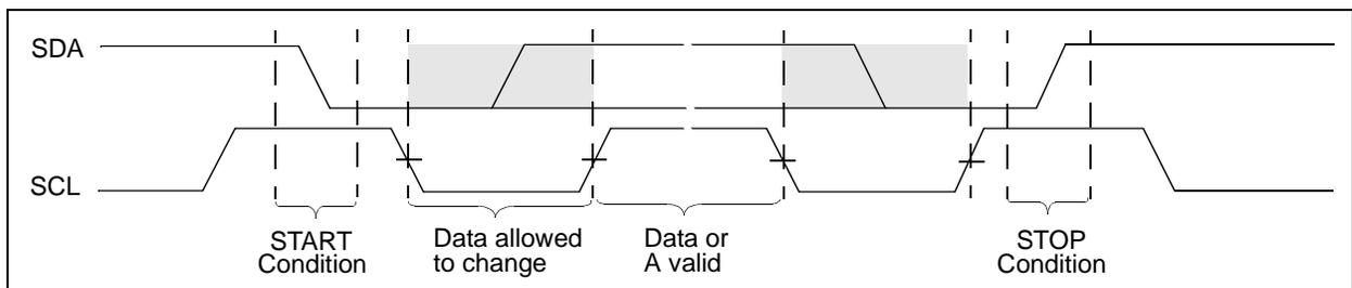
**FIGURE 6-8:** I<sup>2</sup>C Data States and Bit Sequence.
