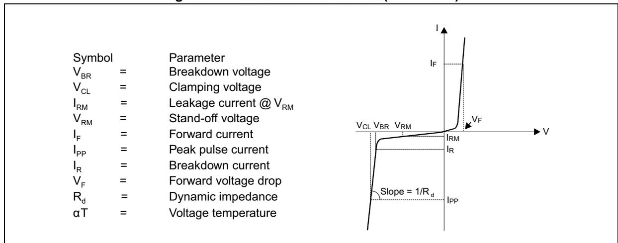
Table 2. Electrical characteristics (values,  $T_{amb} = 25\text{ }^{\circ}\text{C}$ )
