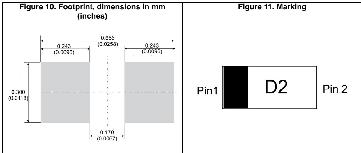
Note: Product marking may be rotated by 180° for assembly plant differentiation. In no case should this product marking be used to orient the component for its placement on a PCB. Only pin 1 mark is to be used for this purpose.
