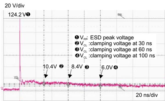
**Figure 6. ESD response to IEC 61000-4-2 (-8 kV contact discharge)**
