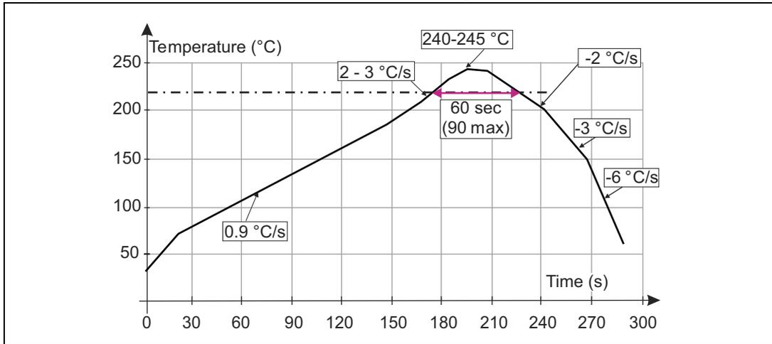
Note: Minimize air convection currents in the reflow oven to avoid component movement. Maximum soldering profile corresponds to the latest IPC/JEDEC J-STD-020.
