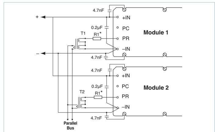
Figure 10 — Transformer-coupled interface
