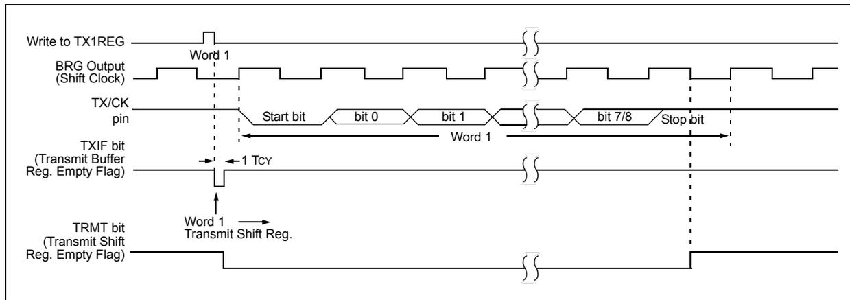
**FIGURE 31-4: ASYNCHRONOUS TRANSMISSION (BACK-TO-BACK)**
