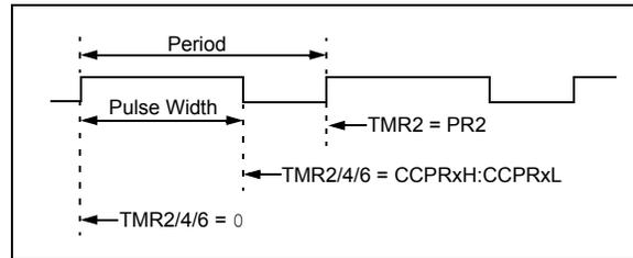
**FIGURE 29-4: SIMPLIFIED PWM BLOCK DIAGRAM**
