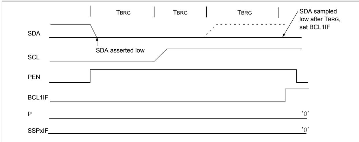
**FIGURE 30-39: BUS COLLISION DURING A STOP CONDITION (CASE 2)**
