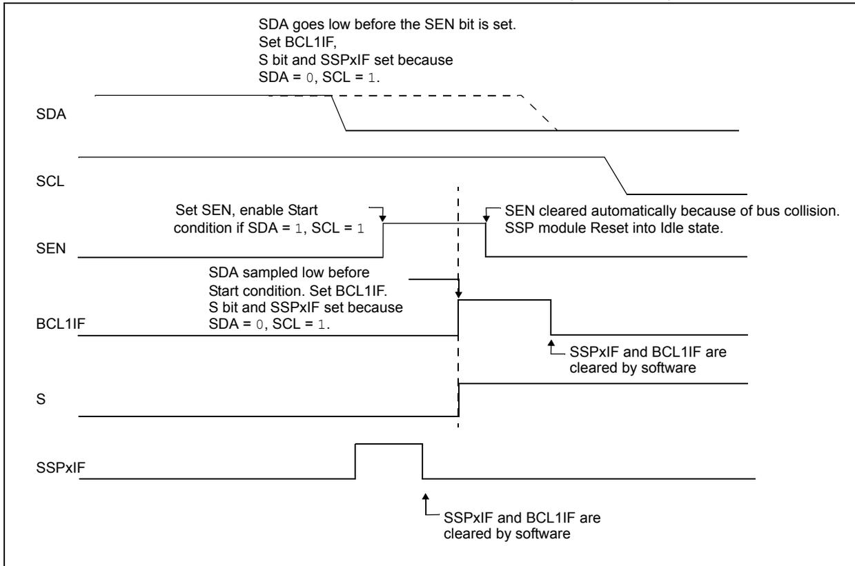
**FIGURE 30-34: BUS COLLISION DURING START CONDITION (SCL = 0)**
