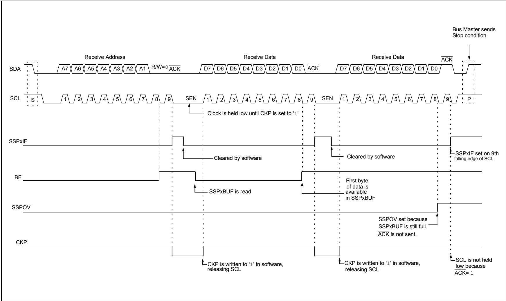
**FIGURE 30-16: I<sup>2</sup>C SLAVE, 7-BIT ADDRESS, RECEPTION (SEN = 0, AHEN = 1, DHEN = 1)**
