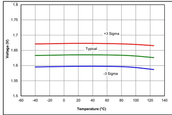
FIGURE 36-110: POR Rearm Voltage, Normal Power Mode
