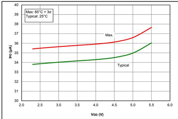
**FIGURE 36-13:**  $I_{PD}$ , Comparator
