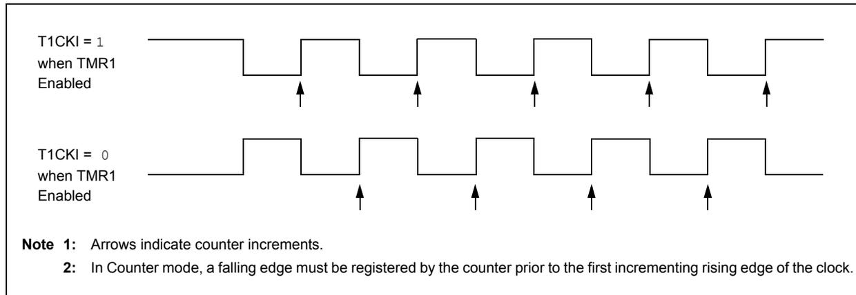
**FIGURE 27-4: TIMER1 GATE ENABLE MODE**
