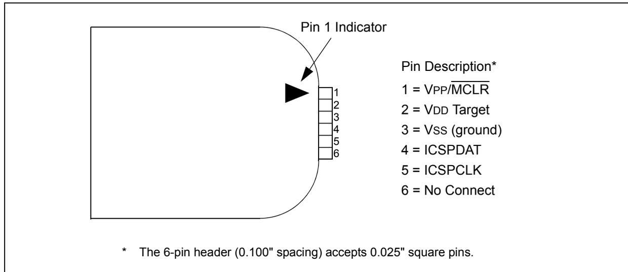
FIGURE 33-3: TYPICAL CONNECTION FOR ICSP™ PROGRAMMING
