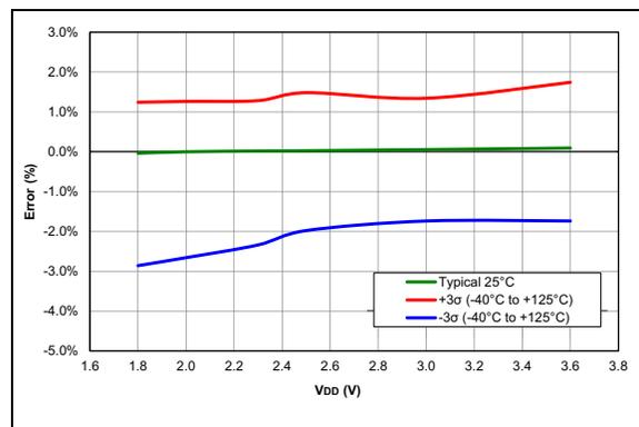
**FIGURE 36-30:** HFINTOSC Typical Frequency Error (PIC16LF18326/46 only)
