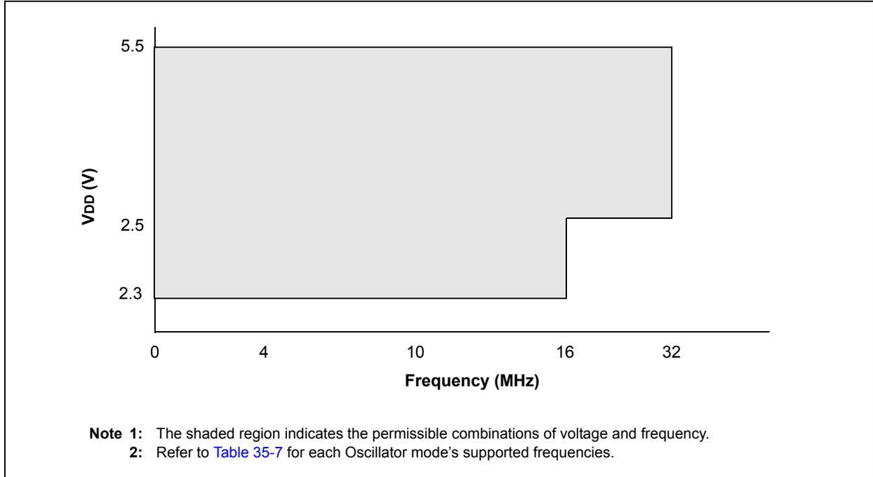
**FIGURE 35-2: VOLTAGE FREQUENCY GRAPH,  $-40^{\circ}\text{C} \leq T_A \leq +125^{\circ}\text{C}$ , PIC16LF18326/18346 ONLY**
