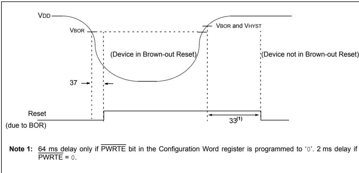
**Note 1:** 64 ms delay only if  $\overline{\text{PWRT}}\text{E}$  bit in the Configuration Word register is programmed to '0'. 2 ms delay if  $\overline{\text{PWRT}}\text{E} = 0$ .
