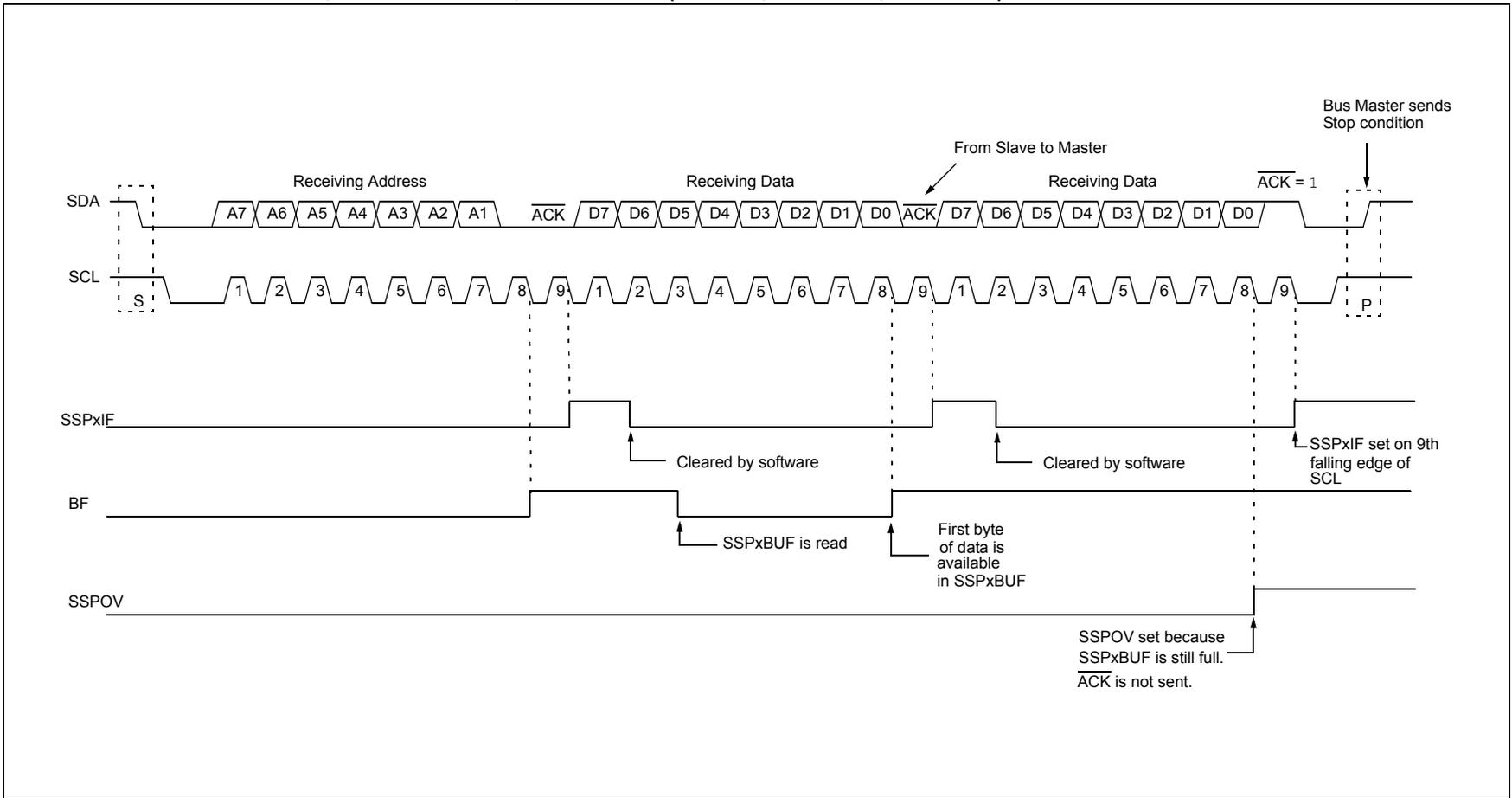
**FIGURE 30-15: I<sup>2</sup>C SLAVE, 7-BIT ADDRESS, RECEPTION (SEN = 1, AHEN = 0, DHEN = 0)**
