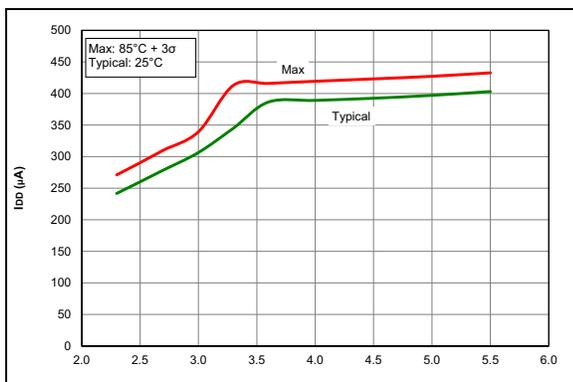
**FIGURE 36-17:**  $I_{DD}$ , XT Oscillator 4 MHz
