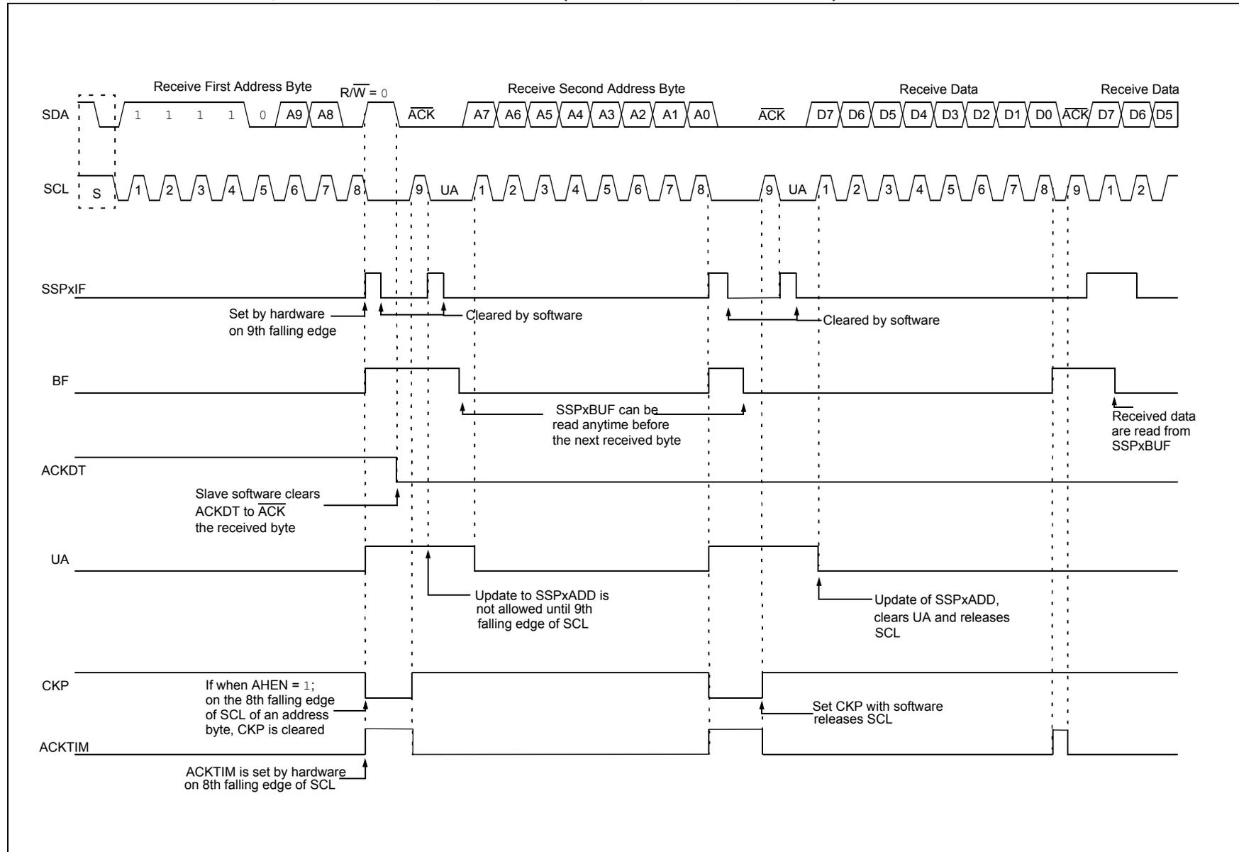
**FIGURE 30-22: I<sup>2</sup>C SLAVE, 10-BIT ADDRESS, TRANSMISSION (SEN = 0, AHEN = 0, DHEN = 0)**
