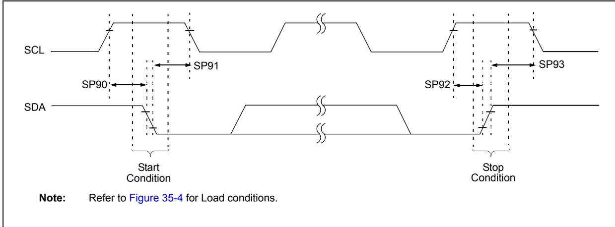
**TABLE 35-23: I<sup>2</sup>C BUS START/STOP BITS CHARACTERISTICS**
