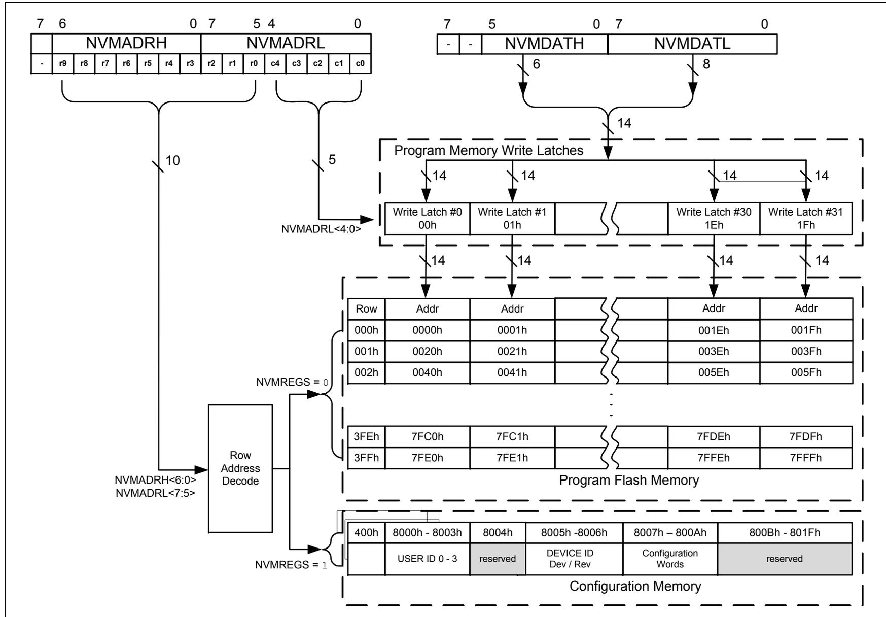
**FIGURE 11-5: PROGRAM FLASH MEMORY WRITE FLOWCHART**
