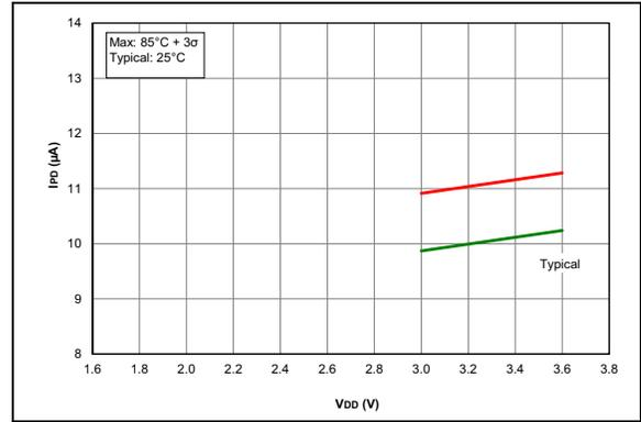
**FIGURE 36-8:**  $I_{PD}$ , Brown-Out Reset (BOR),  $BORV = 1$  (PIC16LF18326/46 only)
