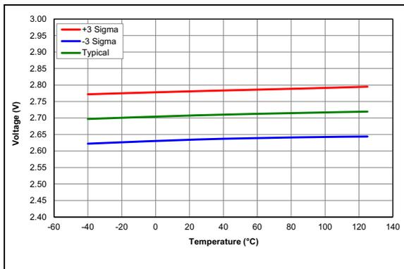
**FIGURE 36-41:** Brown-Out Reset Voltage,
