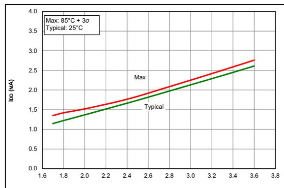
**FIGURE 36-18:**  $I_{DD}$ , HS Oscillator 32 MHz
