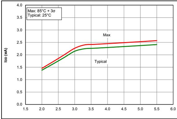
**FIGURE 36-19:**  $I_{DD}$ , HS Oscillator 32 MHz (PIC16F18326/46 only)
