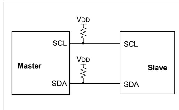
On the last byte of data communicated, the master device may end the transmission by sending a Stop bit. If the master device is in Receive mode, it sends a NACK in place of the last ACK bit. A Stop bit is indicated by a low-to-high transition of the SDA line while the SCL line is held high.
