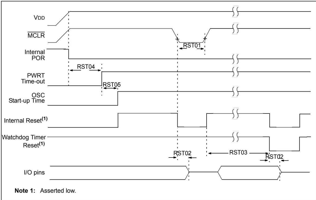
**FIGURE 35-9: BROWN-OUT RESET TIMING AND CHARACTERISTICS**
