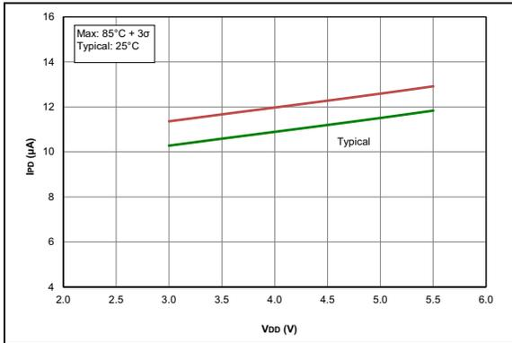
**FIGURE 36-9:**  $I_{PD}$ , Brown-Out Reset (BOR),  $BOVR = 1$  (PIC16F18326/46 only)
