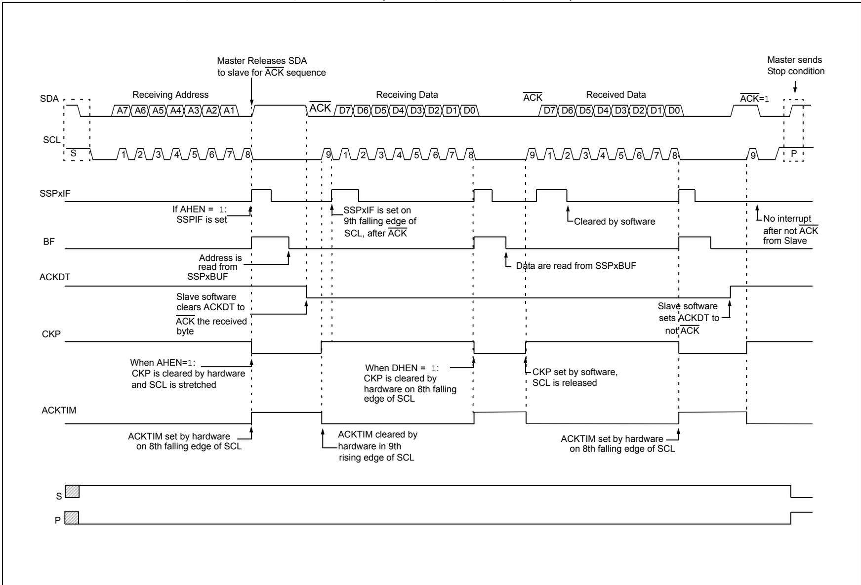
**FIGURE 30-17: I<sup>2</sup>C SLAVE, 7-BIT ADDRESS, RECEPTION (SEN = 1, AHEN = 1, DHEN = 1)**
