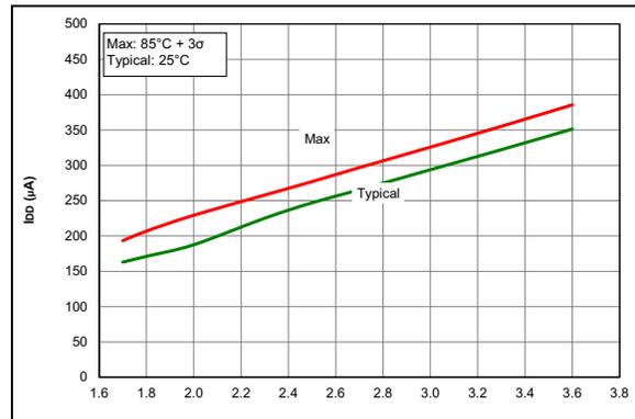
**FIGURE 36-16:**  $I_{DD}$ , XT Oscillator 4 MHz
